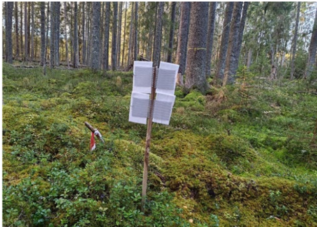
An air filter in a Swedish forest stand for collection of environmental DNA for assessment of biodiversity (photo: Amanda Mikko)
