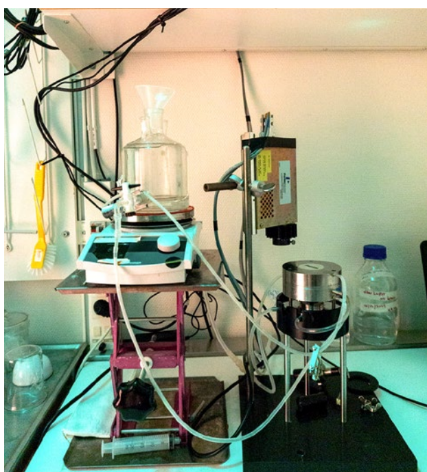
The home-built Joliot-type electrode allows measuring flash-induced oxygen evolution patterns (FIOPs) (photo: Anne Honsel)
