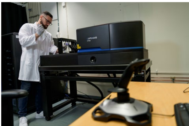
Loading samples to the microfluidics system of the C-Trap (photo: Mattias Pettersson)
